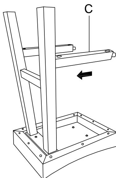
DO NOT TIGHTEN BOLTS UNTIL COMPLETELY ASSEMBLED.
